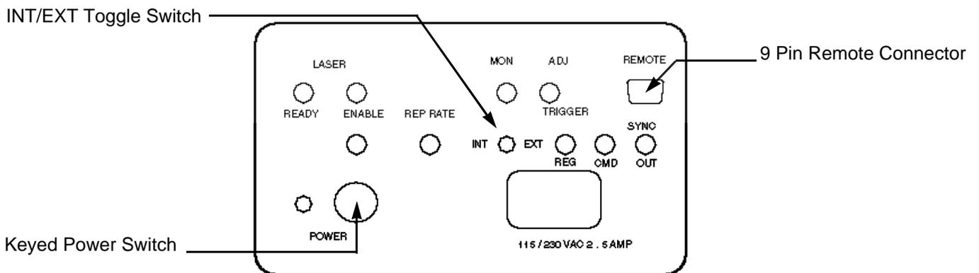
Figure 2 - Laser Control Panel
