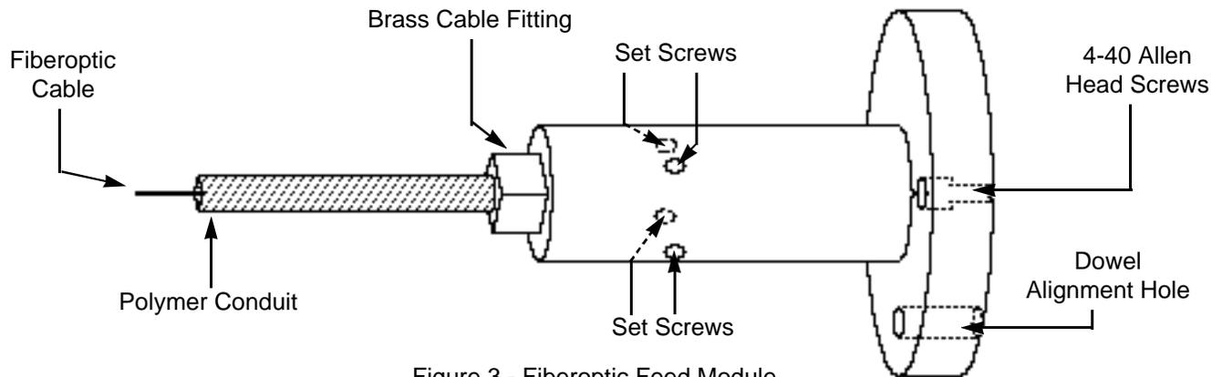
Figure 3 - Fiberoptic Feed Module
